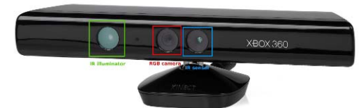
Time of Flight - Kinect
